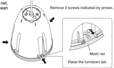
**Step 3.** Clean the speaker cover and mesh net. Wipe with a soft cloth damped in a detergent.
